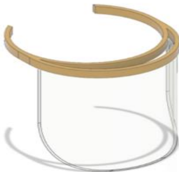
Figure 1. Image of the double arch of the visor and the protective screen.
