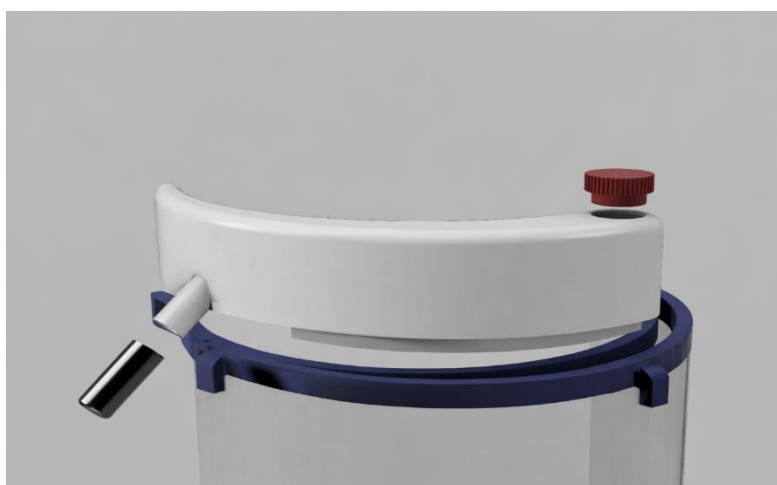
Figure 2. Model of the double-arch frame and the reservoir (detached from the frame).
