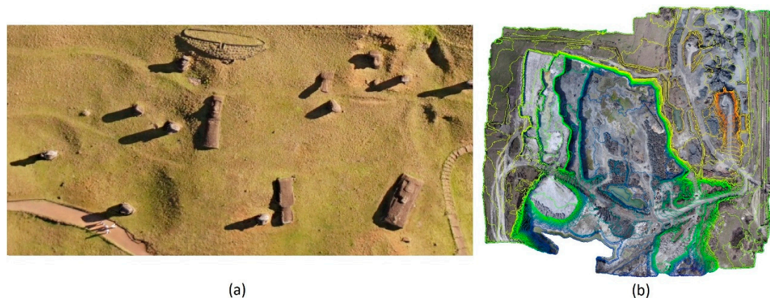
Figure 13. (a) Part of an orthomosaic of Rapa Nui created by UAS photogrammetry; statues' shadows point in different directions since the mosaic combines multiple images taken at different times (source: [31]), (b) Contour
