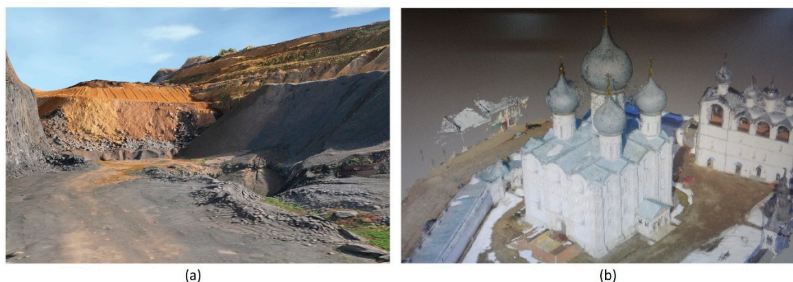
Figure 12. (a) 3D Digital Landscape Model (DLM) of a quarry, i.e. a virtual landscape, generated by draping an orthoimage over a Digital Surface Model (DSM), created from images taken with a camera mounted on a UAS (source: [30]), (b) SGM point cloud of the Cathedral of Rostov-on-Don generated from UAS images (source: [5] (p. 102), courtesy: Racurs, Moscow, Russia).
