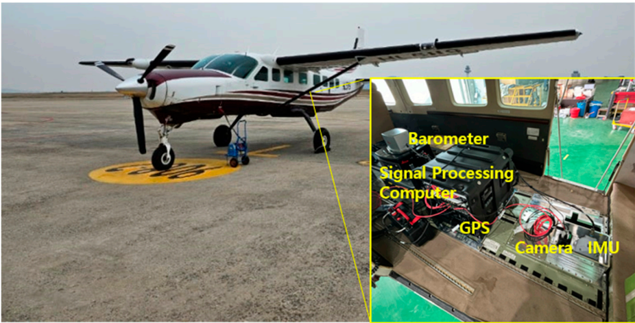
Figure 8. Aircraft used for flight testing, showing onboard sensors (IMU, GNSS receiver, camera, barometric altimeter)
