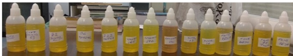
Figure 1. Macroscopic Analysis on color, odor, sediment formation and two- phase separation for 41 marine diesel fuels.
