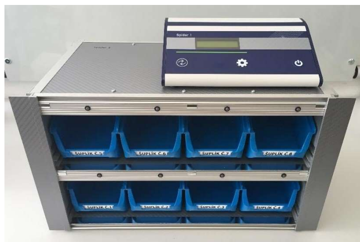
Figure 4. Constructed Pick to Light device labelled Spider 1.
