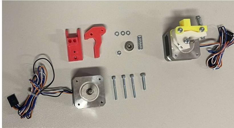
Figure 5. Extruder with motor in unfolded and folded state.
