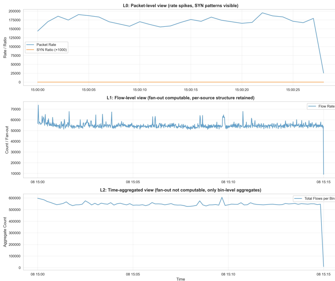
Figure 3. Trace of port-scan-like behavior across evidence layers. L0 shows packet-level rate spikes and SYN patterns; L1 shows per-source fan-out (visible); L2 shows only aggregate counts (fan-out not computable).
