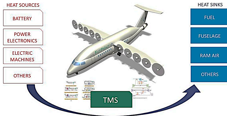
Figure 5. Thermal management system (TMS) of an aircraft with a hybrid power plant [7].
