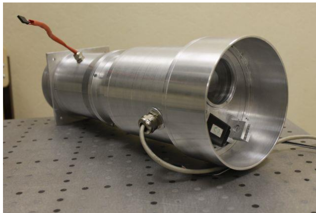
Figure 2. The appearance of the hyperspectrometer (quoted from [1]).
