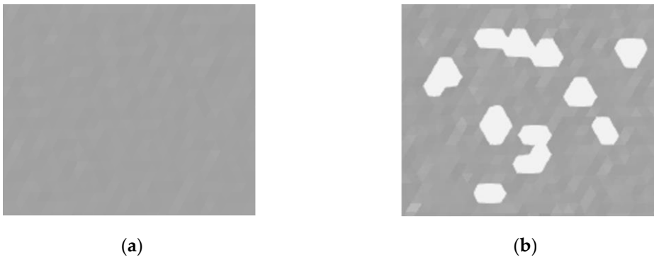
Figure 8. 3D measuring view in ARAMIS® software in an 800 °C environment: (a) Appropriate dot size: smooth and flat and (b) Inappropriate dot size: missing area.
