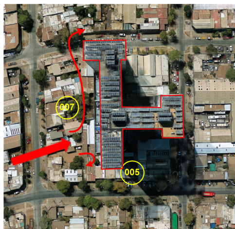
Figure 11. Location of houses 005 and 007 with respect to the building and predominant wind direction.
