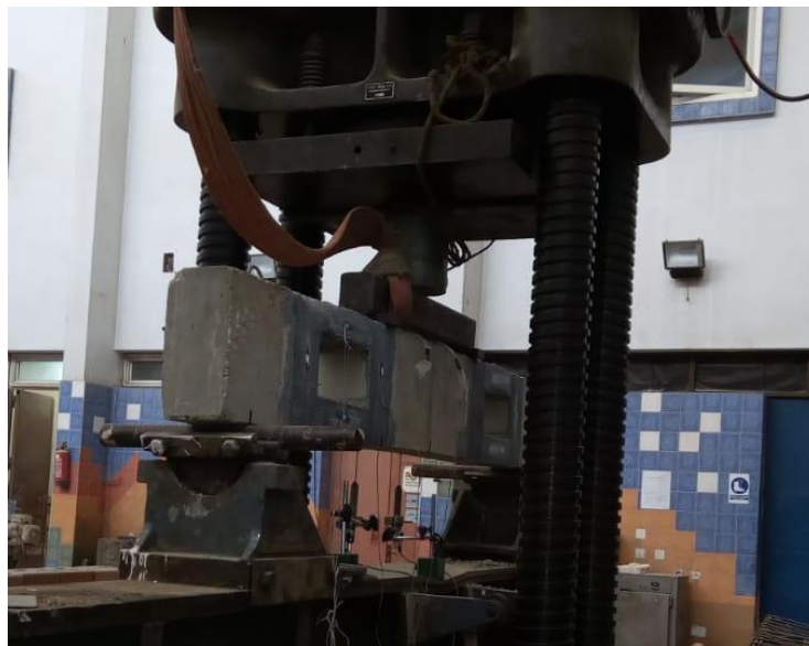
Figure 9. Loading and Test Setup for the tested Beams.
