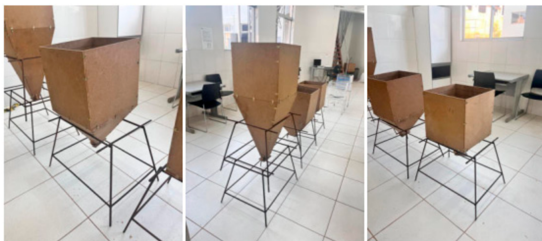
Figure 1. Schematic representation of the reduced-scale prismatic silos and experimental setup.
