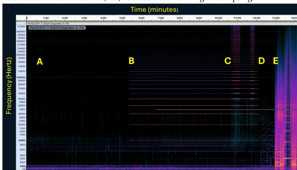
Figure 3. Spectrogram of anaerobic digester treated with sound. A: Background sound levels; B: Digester exposed to a mix of one through five kHz sine waves at one kHz intervals. C: Volume of sine waves increased to one-half to accentuate harmonics; D: Digester exposed to a recording of Neptune, the Mystic from Gustav Holst's orchestral suite The Planets ; E: Digester exposed to a recording of guitar feedback.
