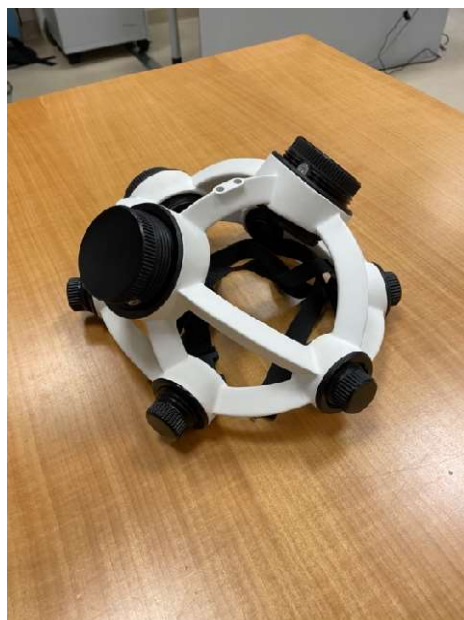
Figure 1. MAGxx1.1 helmet, with Neodymium magnet.
