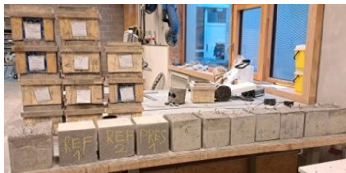
Figure 1. All of the concrete blocks that were prepared using the molds shown on the left.
