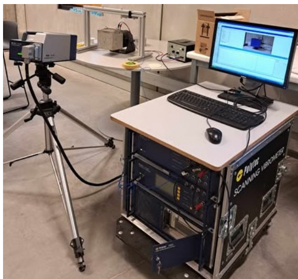
Figure 6. A picture of the PSV-400 laserhead measuring the vibration of the concrete block from the BRÜEL & KJÆR Vibration Exciter
