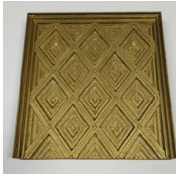
Figure 24. Mockup of the coffered ceiling with golden finish.
