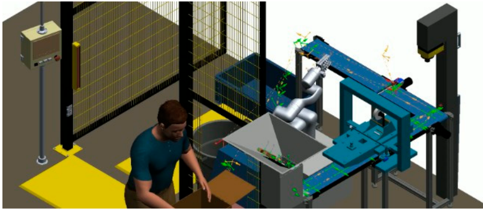
Figure 9. Automated system implemented in Process Simulate.
