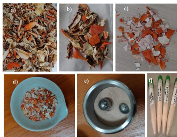
Figure 1. Images of the sample appearance during the steps performed for processing the raw material, represented by the aged biogenic waste: a), b) Cooked crab shell before and after selecting suitable fragments; c) cleaned raw material; d) Cleaned and mechanically crushed material; e) Biogenic powder obtained through the ball milling process; f) obtained powder samples.
