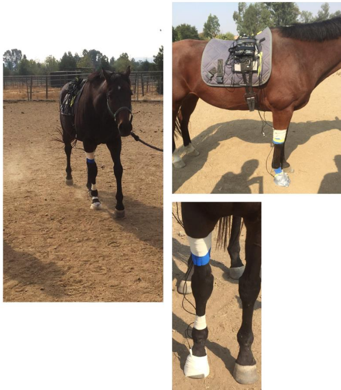
Figure 3. Test of AMG measurements simultaneously from the hoof wall and frog. Left image; a horse equipped with AMG sensors walking whilst being recorded. Upper right image; the CURO MkI setup with WiFi unit on the girth and cables to the sensors. Lower right image; a close up on the limb being measured showing the use of tape and Snøgg to hold the cables and sensors in place during recordings.
