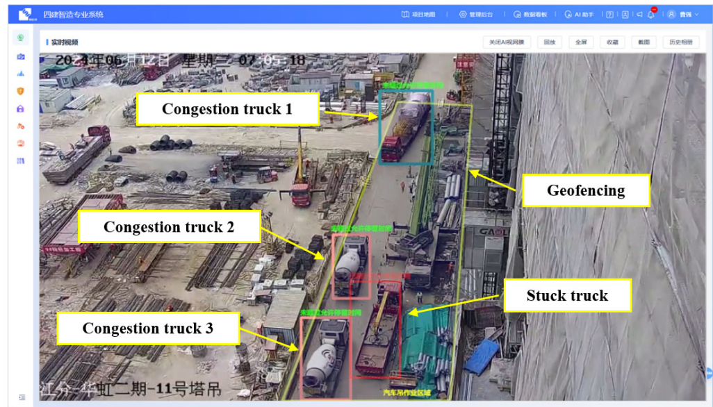
Figure 5. Example of geofencing and congestion prediction.
