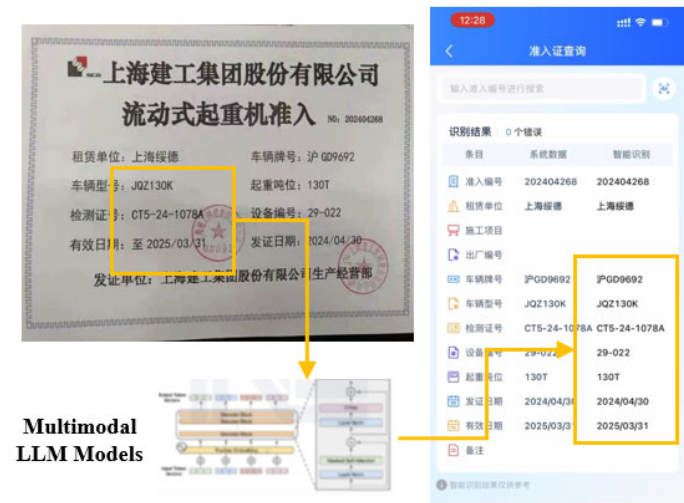
Figure 6. Crane permit verification based on MLLM.
