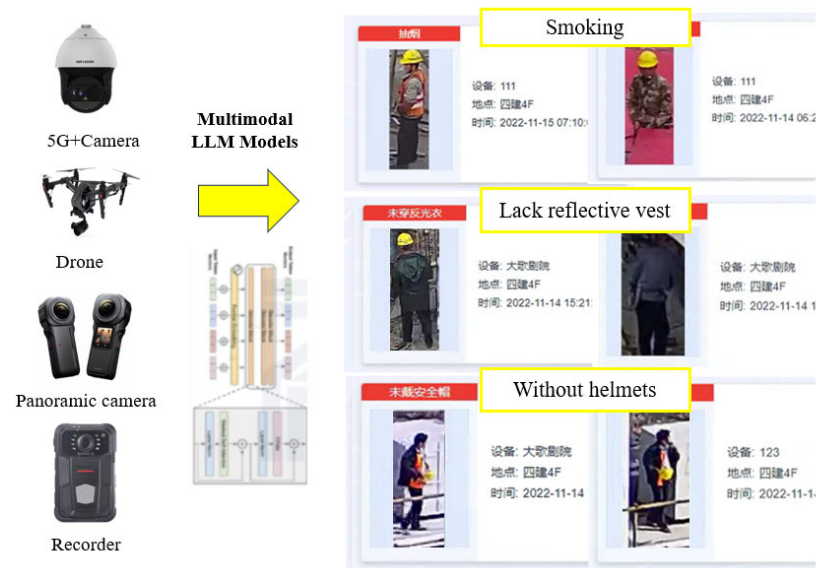
Figure 4. AI-driven behavior detection using MLLM.
