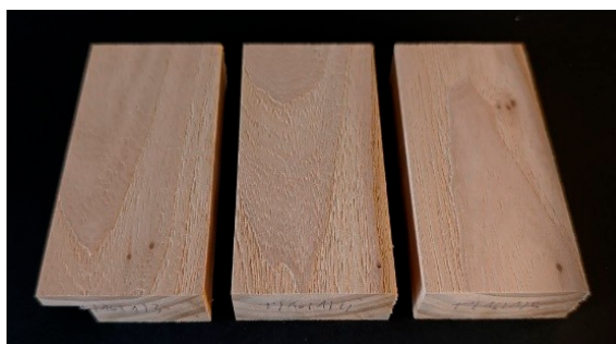
Figure 3. Tangential surfaces of sandblasted elm wood.
