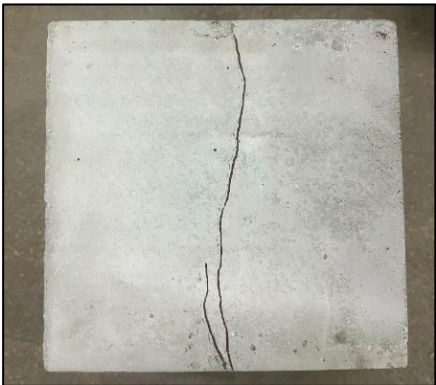
Figure 6. Crack development after splitting.
