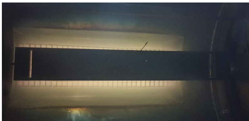
Figure 5. Photo of the process chamber with fast-neutrals source and sample holder.
