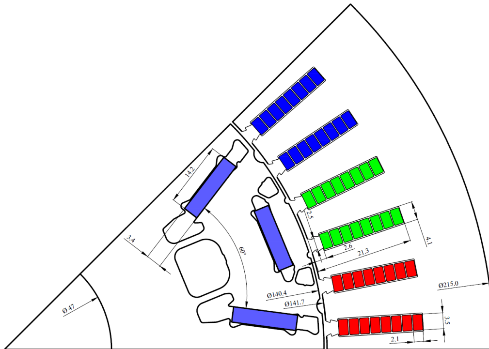
Figure 4. Machine geometry - detailed view of one pole.
