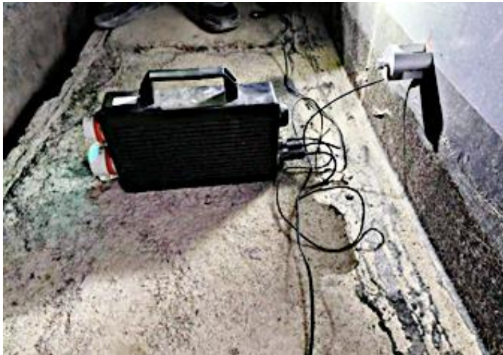
Figure 6. On-site installation diagram for a piezoelectric ceramic sensor.
