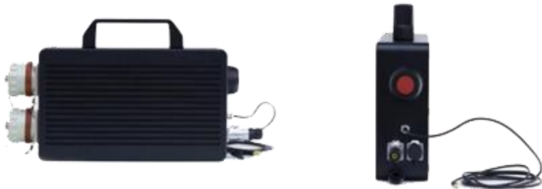
Figure 3. Explosion-proof acoustic emission instrument.
