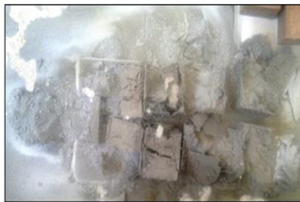
Figure 6. Effect of ZnO NPs on cube cement pastes at curing water.
