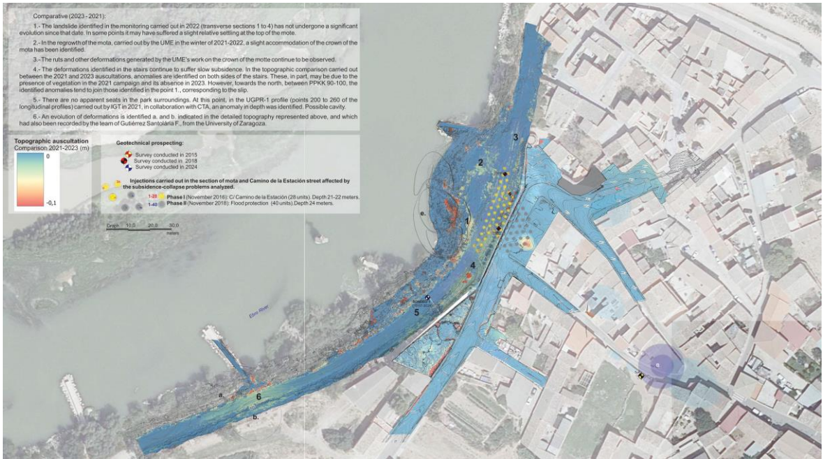
Figure 7. Topographic comparison between the data obtained on November 22, 2021, and November 5, 2023. Obtained with the RTC360 laser scanner. General situation plan.
