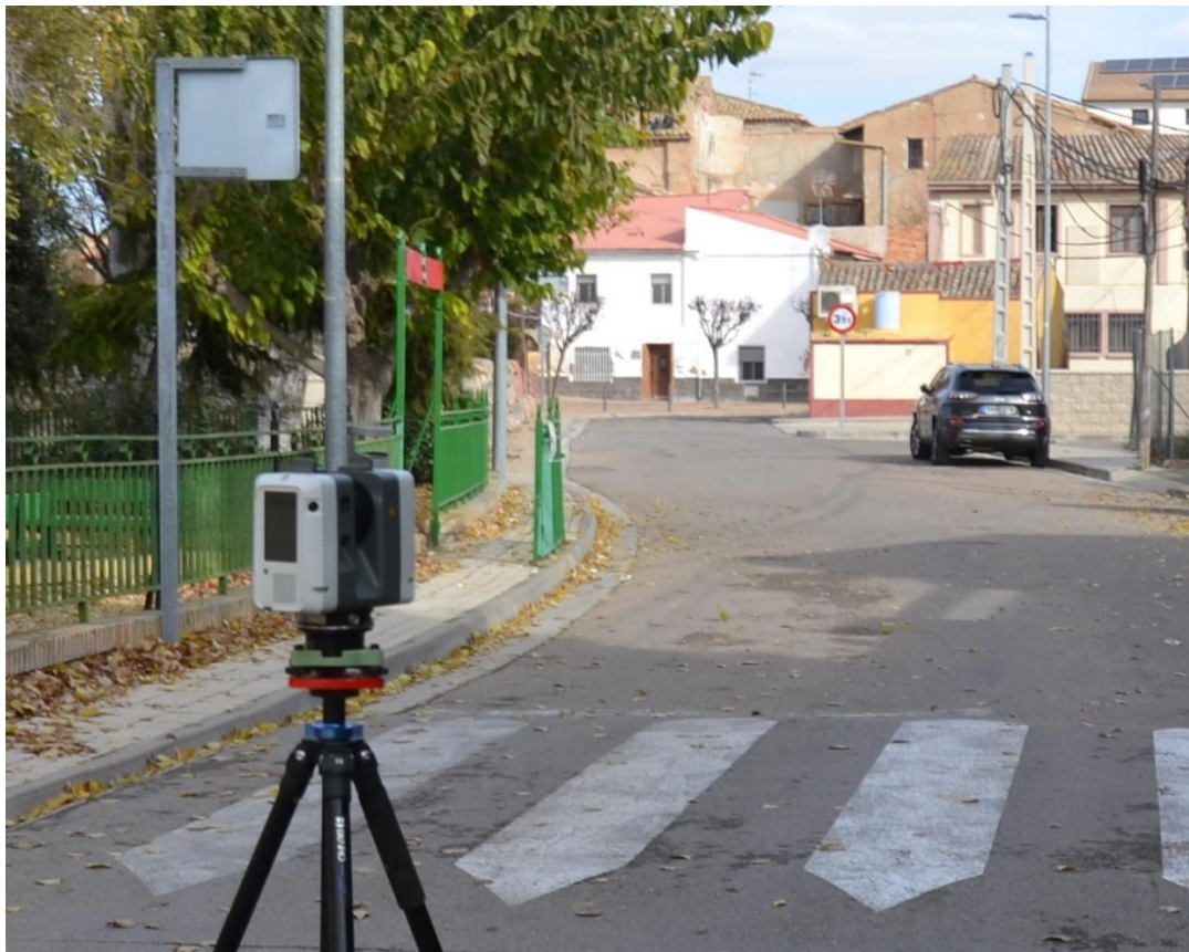
Figure 5. RTC360 laser scanner during topographic auscultation work.
