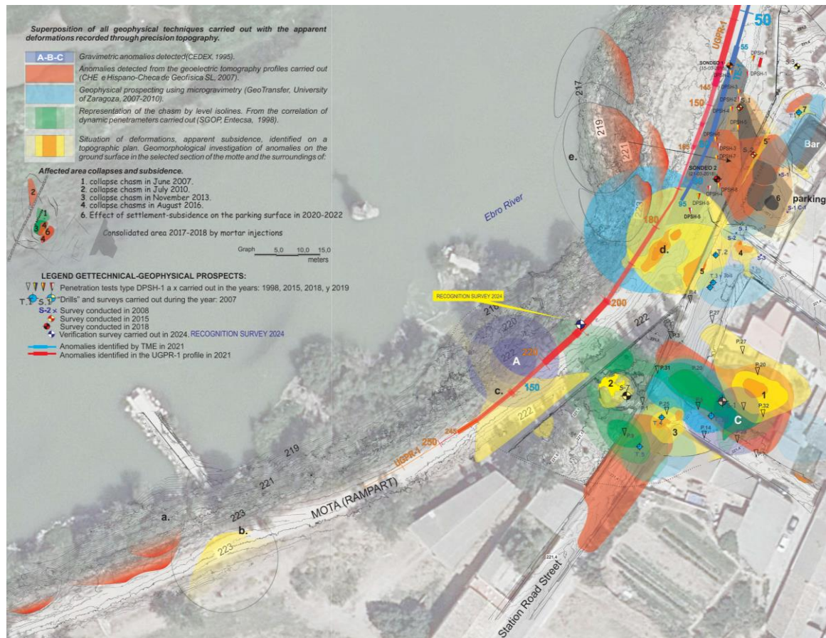
Figure 9. Zoning obtained with the anomalies observed in the detailed topography carried out and the different geophysical prospecting campaigns.
