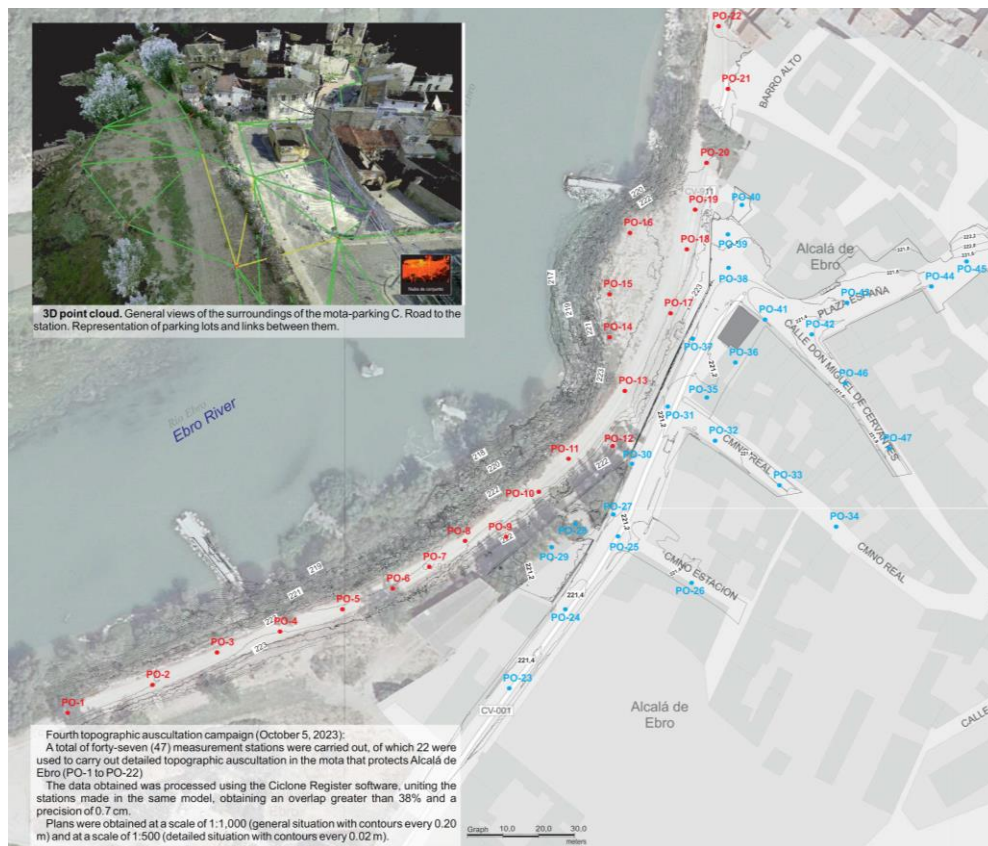
Figure 6. Measuring stations used for topographical auscultation. 24 at the moat (red colour) and 27 in the village (blue colour). Result of the precision achieved in September 2024.
