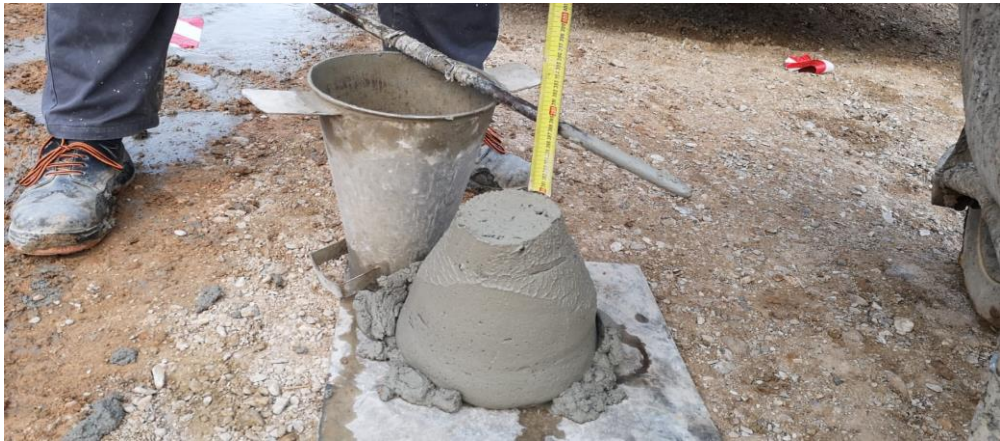
Figure 3. Control of the consistency of the mortar B.M. Abrams cone between 8 and 12 cm.
