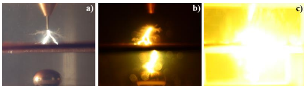
Figure 6. Example photos of discharges in point to sphere electrode system with a pressboard barrier, where: a) discharge develops between HV point and barrier, b) discharge develops on both sides of barrier, c) breakdown.
