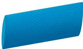
Figure 15. Textured NACA0015 blade with surface embossing for self-starting enhancement, as investigated by Seifi et al. [7].
