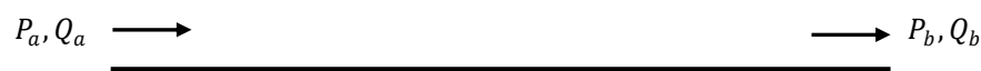
Figure 1. Schematic of a fluid transmission line with the input and output variables.
