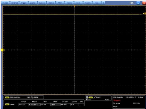
(a) Time domain waveform of voltage before voltage regulation
