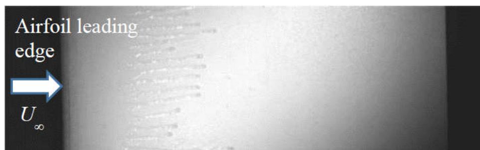
Figure 2. Experimental study to examine surface water runback over an ice accreting airfoil(Waldman, Liu et al. 2015).
