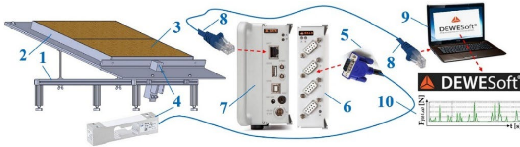
Figure 6. Measuring chain using DS NET to sense tensile force F_{M(\delta_1),k} [N]. 1 – laboratory device, 2 – PLEXI frame, 3 – bulk material, 4 – load sensor [52], 5 – D-Sub plug, 6 – BR4-D measuring module [11], 7 – gateway module DS GATE [53], 8 – network cable, 9 – laptop, 10 – DEWESoft X2 SP5 software [54].
