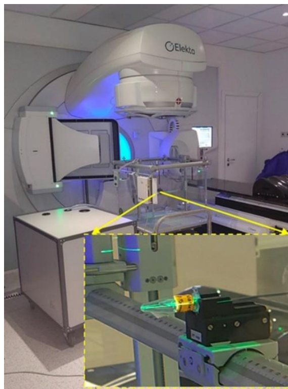
Figure 3. Image of the LINAC suite used for enzyme solution irradiation. The inset shows a close-up of the sample support positioned within the water phantom.
