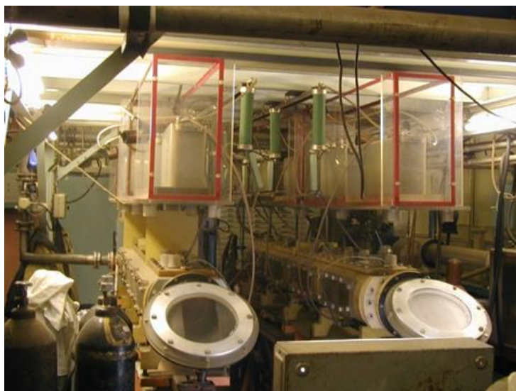
Figure 5. Experimental setup for studying the characteristics of pulsed electric discharge CO 2 lasers and the effect of their radiation on materials. Laser cuvettes with Brewster windows made of NaCl single crystals with a diameter of 300 mm [5,81].
