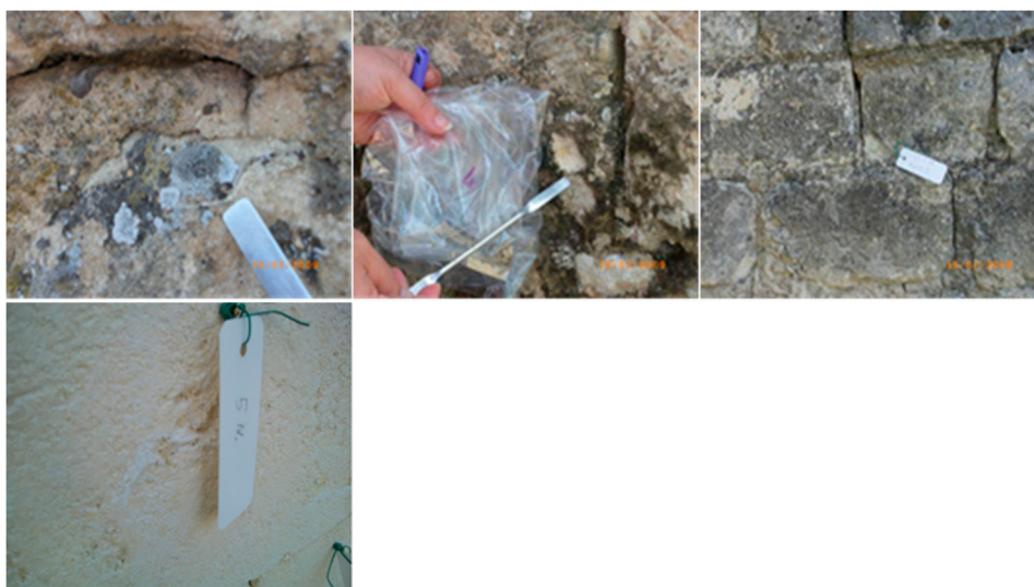
Figure 2. The sampling modalities: a) collection and b) storage of samples; cataloguing: c) on the North East walls of the old farmhouse and d) on the North wall of the new cube in calcarenite.
