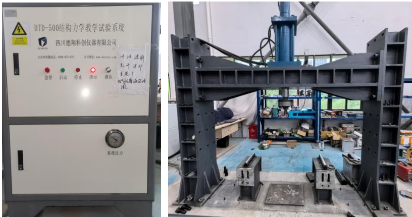
Figure 5-3. DTD-500 structural mechanics experimental equipment.
