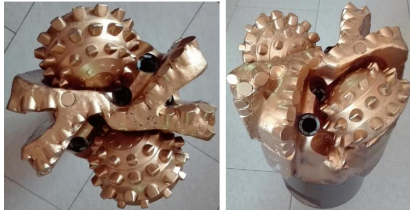
Figure 1. PDC-cone hybrid bit.
