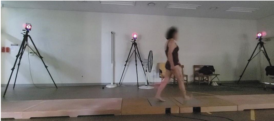
Figure 2. 3D motion capture system and 6-m walkway.
