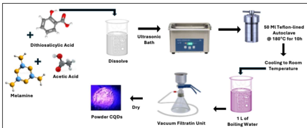
Figure 1. Schematic diagram for the synthesis of carbon quantum dots by Solvothermal method.
