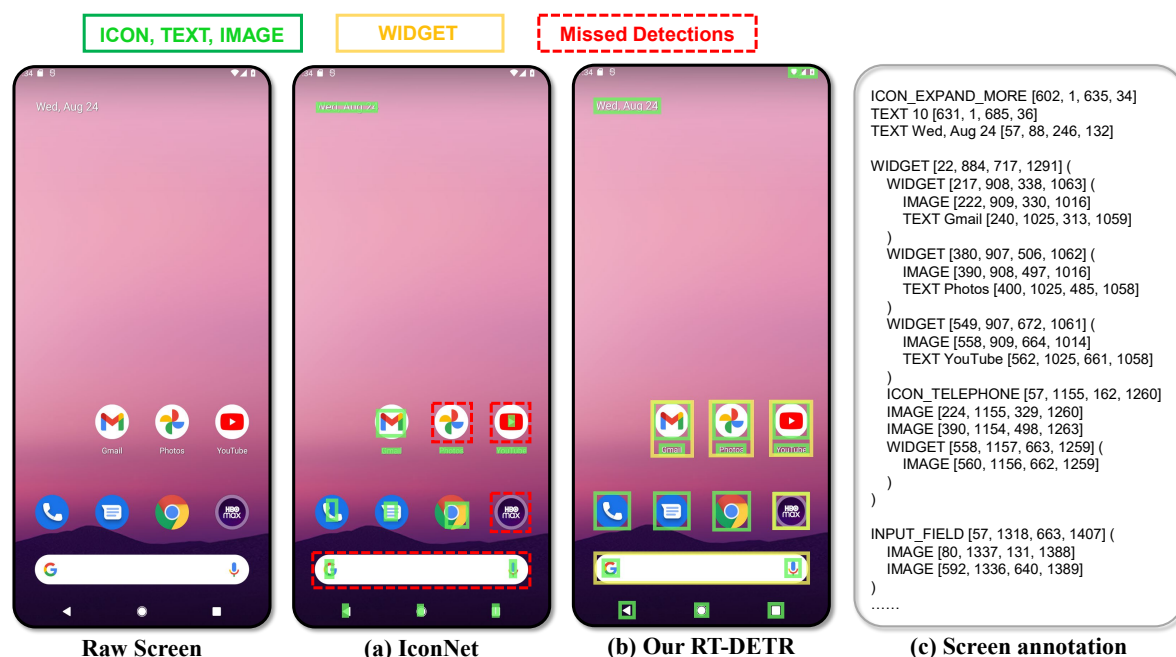
Figure A1. Comparison of different detection models. (a) The detection outcomes from IconNet [42]. (b) The detection outcomes from RT-DETR model trained by us. (c) The corresponding screen annotation example.
