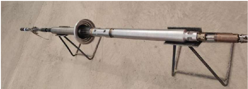
Figure 1. The forty-arm caliper logging tool used in this study.
