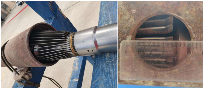
Figure 5. Eccentric passage of the caliper logging tool through the casing and holes used in this study.
