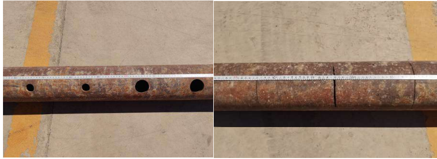
Figure 3. Images of artificially-made holes and cracks used in this study.
