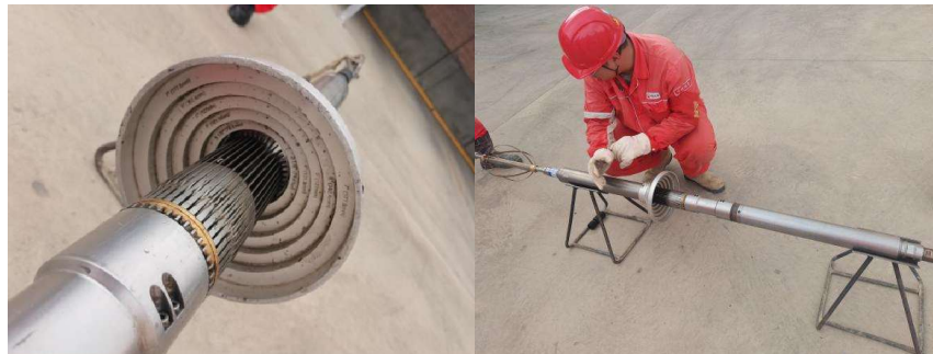
Figure 4. Calibration of the multi-caliper logging tool used in this study.
