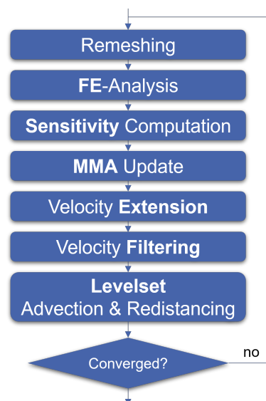
Figure 4. Structure of the optimization loop with the individual components.
