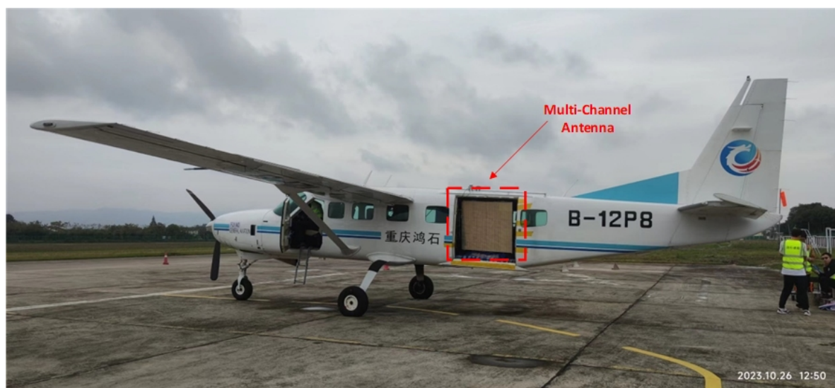
Figure 8. Airplane mounted with multi-channel SAR system.
