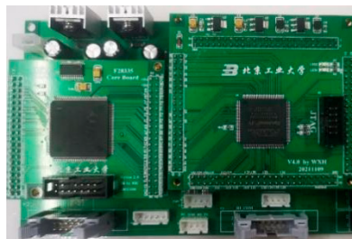
Figure 38. Phase control system.
