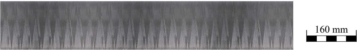
Figure 5. Surface scan of the composite pressure vessel acquired with a line-scan camera.
