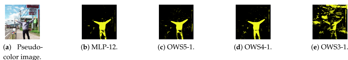
Figure 20. Examples of inference results from some Wavelength Sets models with different band counts (12, 5, 4, and 3). Models with \geq 4 bands perform well. (a) Pseudo-color image. (b) 12-band Multi-Layer Perceptron (MLP-12). (c) 5-band Optimal Wavelength Set (OWS5-1) MLP. (d) 4-band OWS4-1 MLP. (e) 3-band OWS3-1 MLP.
