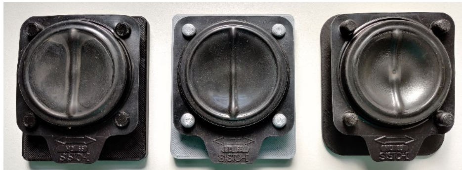
Figure 2. An unused diaphragm (center) with two additional diaphragms exhibiting various wear patterns.
