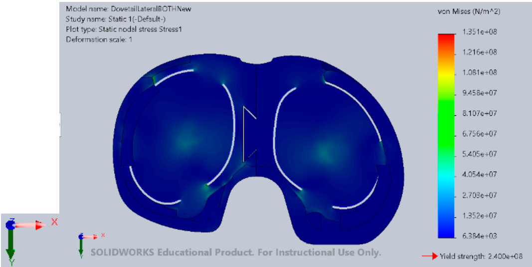
Figure 14. Stress distributions (stress raises at tabs).
