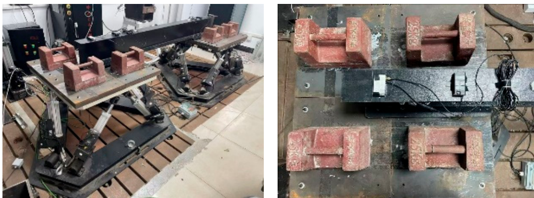
Figure 7. Synchronous vibration test setup for the rigid-connected dual-table array. (a) Dual-table array loading test system (b) Single table load and connection configuration.
