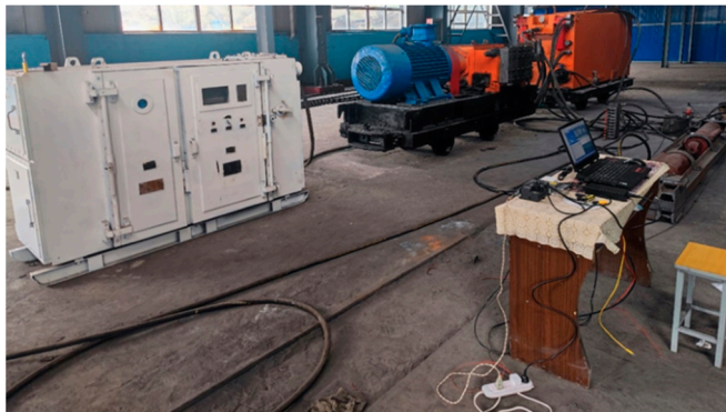
(a) Hydraulic bracket simulation test bench
